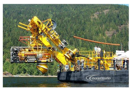
for manned deep submergence systems (NAVSEA P9290), the PRMS is designed, built and tested to exacting standards and represents a quantum step forward in submarine rescue technology.
