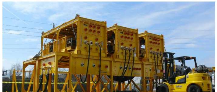
Figure 2 SDFS Battery/Pumping Skids
