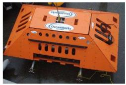
The Shallow Node Pod, designed and built by OceanWorks to provide power and fiber optic communications to "plug and play" scientific
