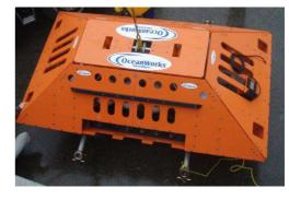
resistant frame (TRF) located near the mouth of the Fraser River at a depth of 170m. This node was connected to 40 km of cable providing power and data path back to the shore station at Iona Point. Engineers at the shore station then brought the system on-line by switching power on to the subsea cable. Instrument packages, with an OceanWorks Science Instrument Interface Module (SIIM), were then deployed at the node.
