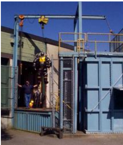
Tank Equipment 3 Ton Hoist
