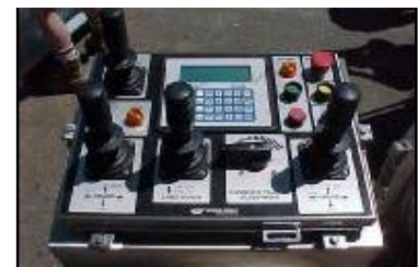
Remote LARS Control Panel
