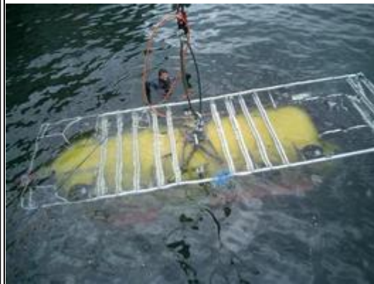
The pressurized rescue Module undergoing initial stability and buoyancy testing in Vancouver, Canada
