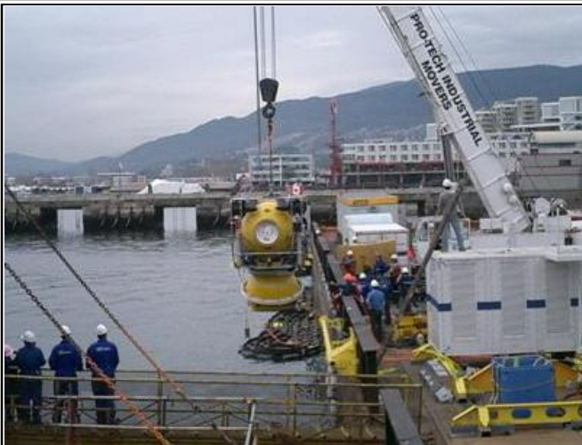
The pressurized rescue Module being lowered into the water for initial pier side testing in Vancouver, Canada
