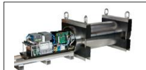
Closing a NEPTUNE Junction Box (Credit: Oceanworks)
